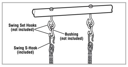
• Fasten the swing S-hooks (included) onto the swing set hooks (not included).
